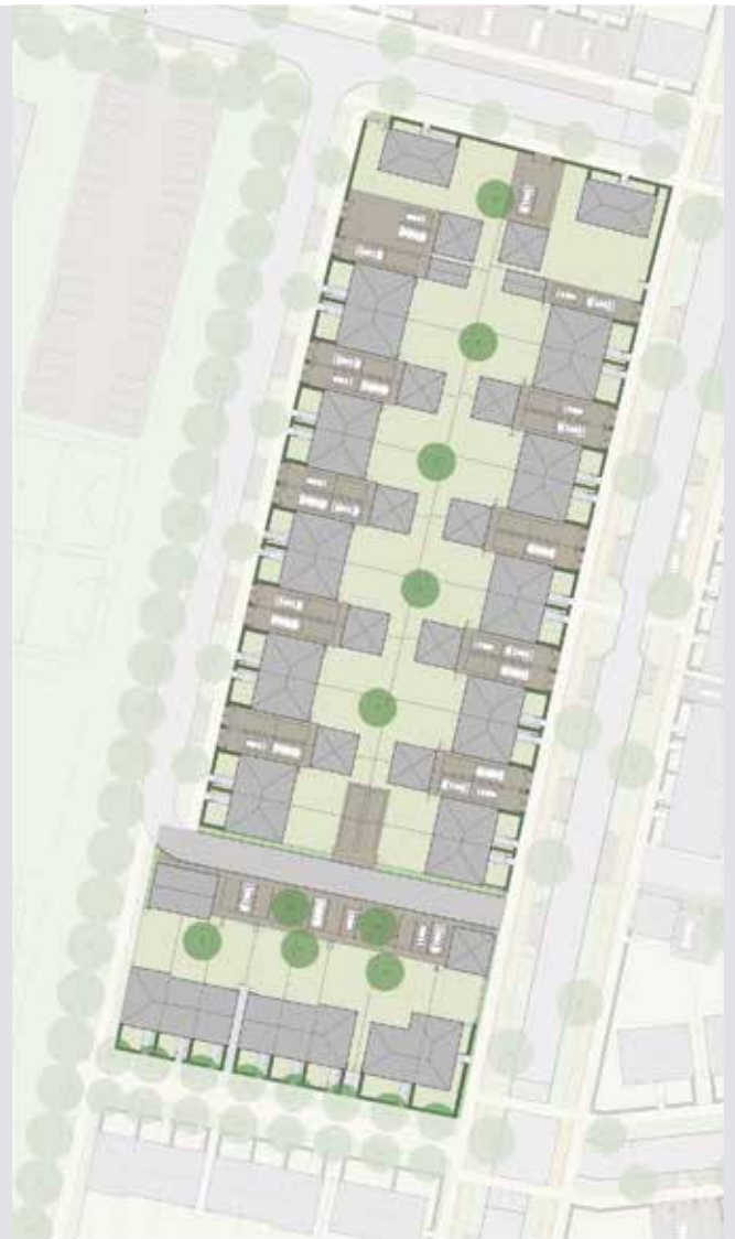
Above: Plan showing a typical back-to-back garden perimeter block; Below: Section through a typical back-to-back garden perimeter block
