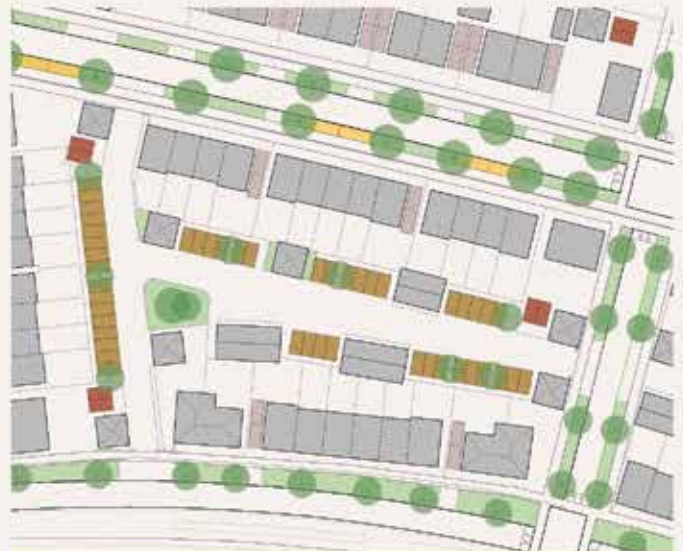
Typical courtyard block with rear-access parking
