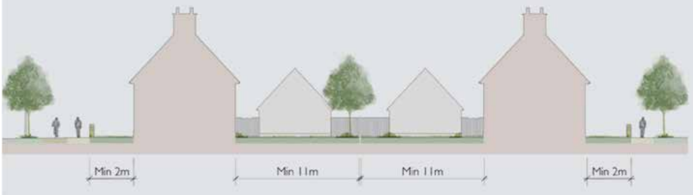
Above: Plan showing a typical back-to-back garden perimeter block; Below: Section through a typical back-to-back garden perimeter block
