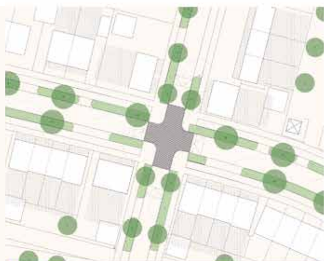
Raised junction at a cross-roads that shall act as a traffic calming feature
