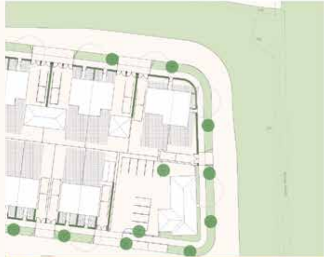
Road alignment with reduced forward visibility that will promote slower vehicle speeds
