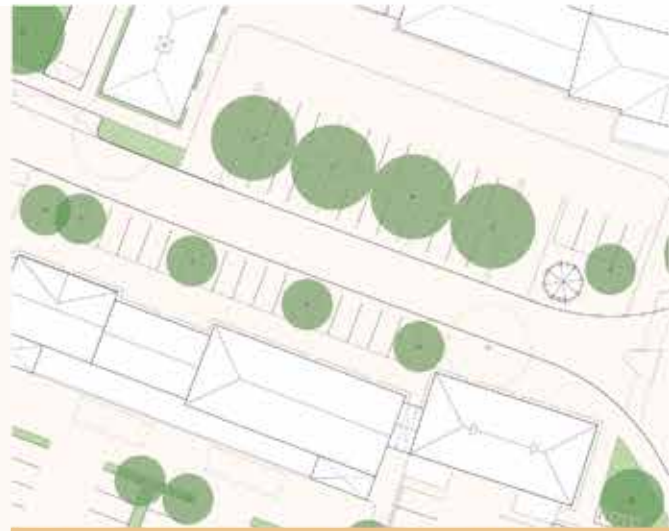
Perpendicular parking at a proposed public space that will function as a traffic calming feature
