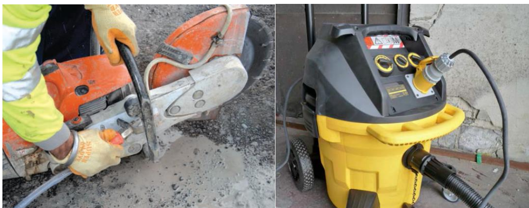
Figure 3-6 Left - Water suppression of a cut-off saw, Right – Example dust extraction unit
