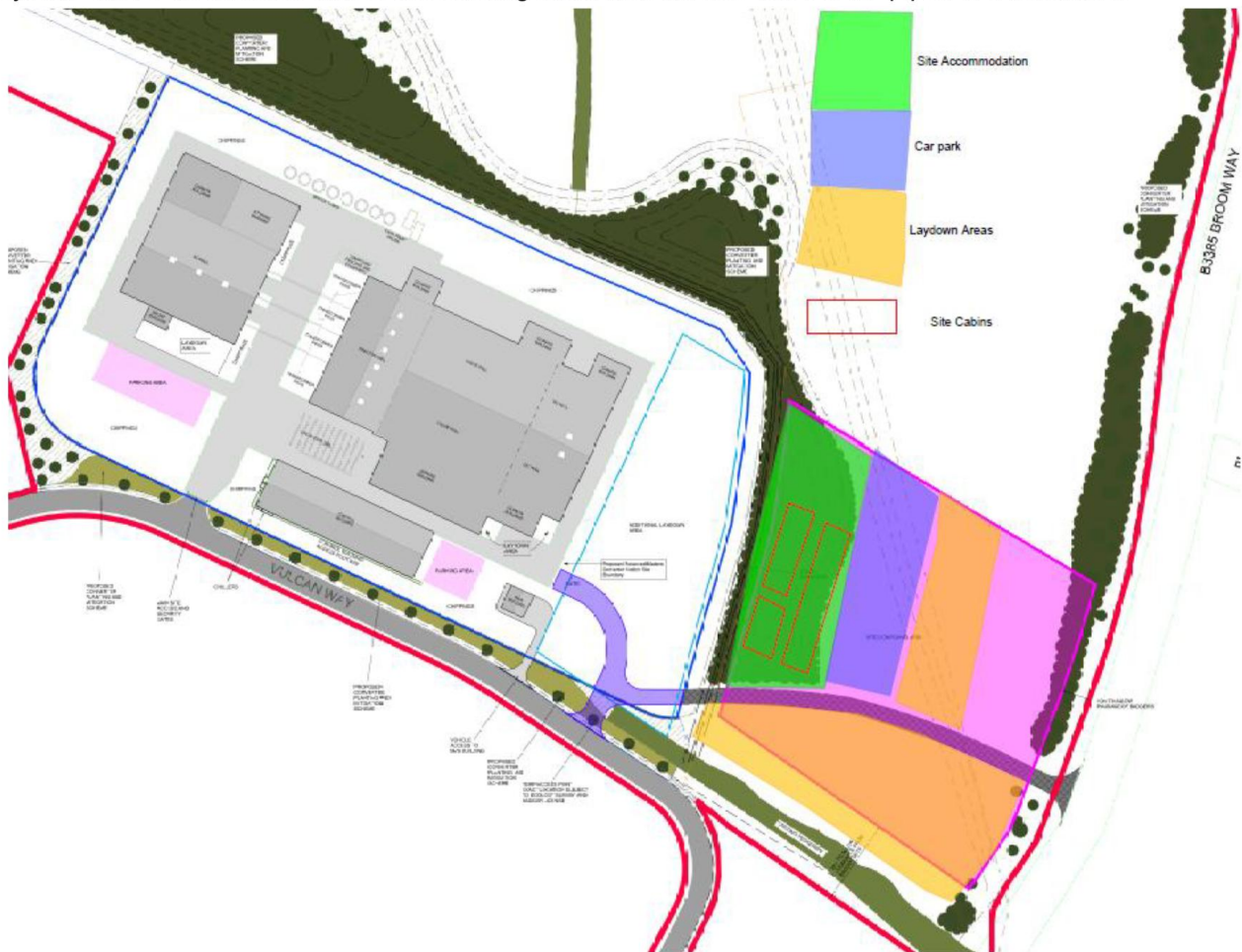
Site Compound, Car Park and Laydown Area
