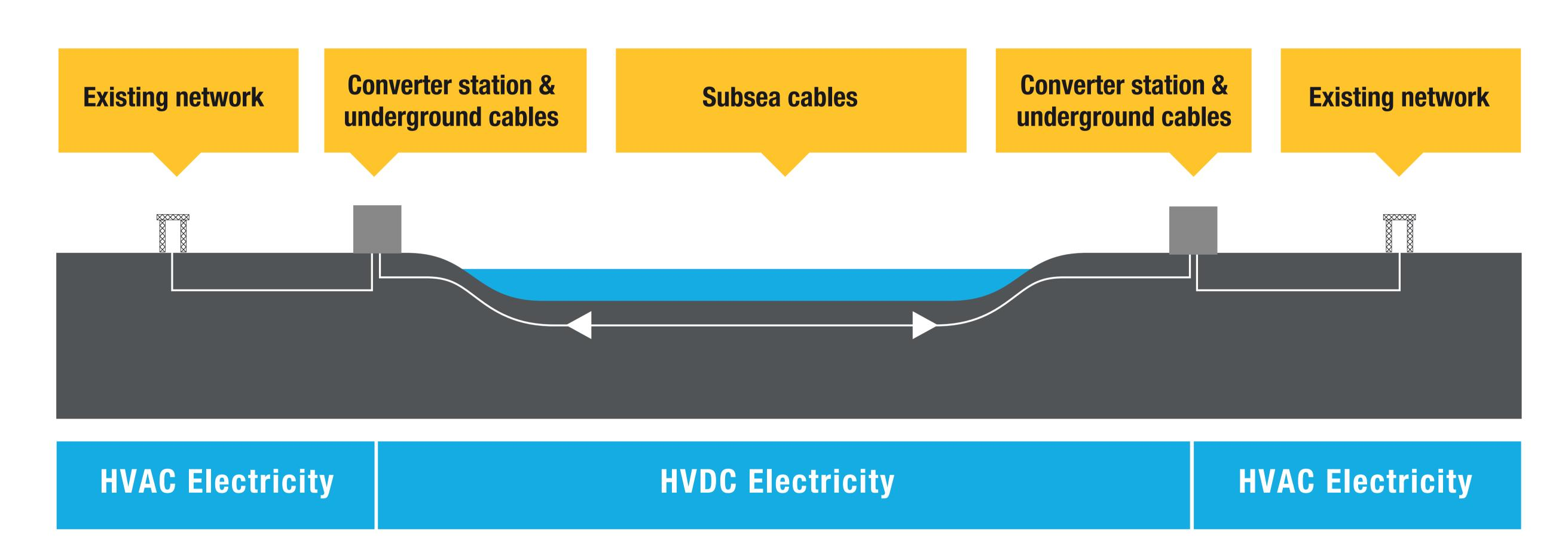
Being an island, Great Britain requires connections with other countries to be made using subsea cables. Differences between electricity transmission in Great Britain and continental Europe, as well as the distances involved, require using high voltage direct current HVDC.
