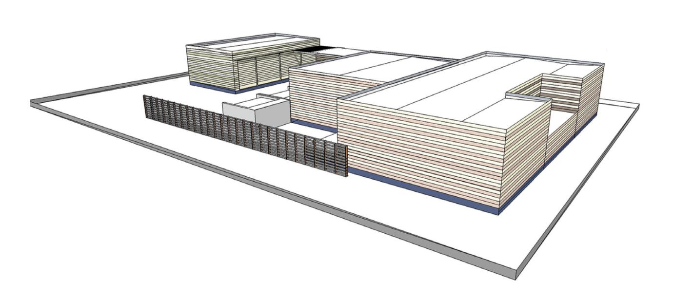
The effects of the converter station on the landscape and on views will be mitigated by appropriate architectural treatment, particularly the ways in which the outsides of the buildings are clad or finished taking note of existing buildings in the surroundings.
