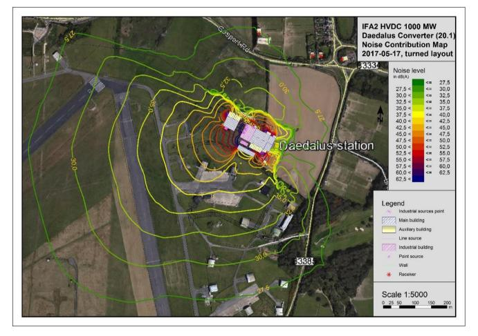
Figure 4 - Noise contribution from the Daedalus converter station, noise levels at 2 m above ground
