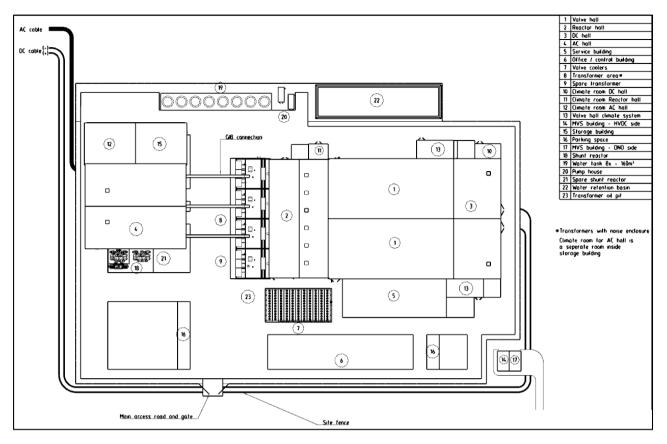
Figure 1- Detailed equipment layout of Daedalus HVDC station
